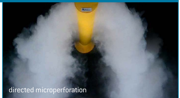
Examples of airflow patterns created using smoke tests in the PRIHODA R&D centre
